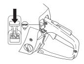
Stop the engine by switching off the ignition.
