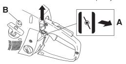
**Decompression valve (C):** Press the valve to reduce the pressure in the cylinder and make starting easier. You should always use the decompression valve when starting the machine. Once the machine has started the valve will automatically return to its original setting.
