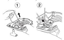
Undo the screw in the centre of the pulley and remove the pulley. Insert and fasten a new starter cord to the pulley. Wind approx. 3 turns of the starter cord onto the pulley. Connect the pulley to the recoil spring so that the end of the spring engages in the pulley. Fit the screw in the centre of the pulley. Insert the starter cord through the hole in the starter housing and the starter handle. Make a secure knot in the end of the starter cord.
