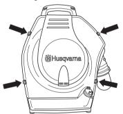
Loosen the two fasteners holding the air filter cowling and remove the filter. Wash the filter clean in warm, soapy water.
