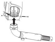
Also pay attention to the stops located on the pipe bend and the fan's outlet pipe. Ensure that the stop on the pipe bend comes in front of the stop on the outlet pipe.
