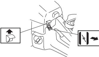
If the machine is fitted with an air purge (A): Press the air purge repeatedly until fuel begins to fill the bulb. The bulb need not be completely filled.
