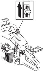
When the switch is pushed upwards, the heat is switched on. When the switch is pushed downwards, the heat is switched off.
