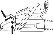
Note! Pull the front hand guard towards the front handle. The chain brake is now disengaged. Your saw is ready for use.
