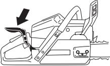
**Never carry or hang the saw by the trigger! This could damage the mechanism and disable the chain brake.**
