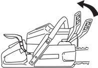
Remove the bar nuts and remove the clutch cover (chain brake). Take off the transportation ring (A).
