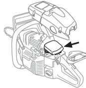
The filter can be cleaned more thoroughly by washing it in water and detergent.
