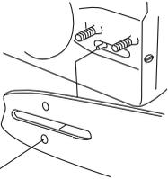
Tension the chain by turning the wheel down (+). The chain should be tensioned until it does not sag from the underside of the bar.
