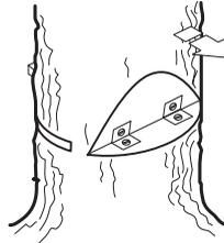
All control over the felling direction is lost if the felling hinge is too narrow or non-existent, or if the directional cuts and felling cut are badly placed.
