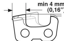
When the length of the cutting teeth has worn down to only 4 mm the chain must be replaced.
