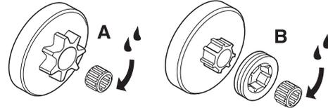
Both versions have a needle bearing on the drive shaft, which has to be greased regularly (once a week). CAUTION! Use only high quality bearing grease or engine oil.
