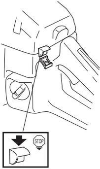
Stop the engine by switching off the ignition.
