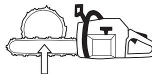
Finish by cutting from above so that the two cuts meet.
