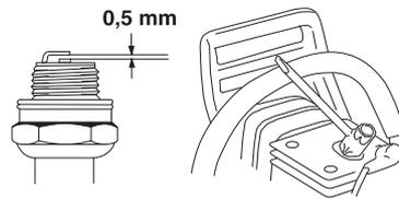
**CAUTION!** Always use the recommended spark plug type! Use of the wrong spark plug can damage the piston/cylinder.
