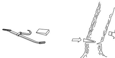
We recommend that you use a bar that is longer than the diameter of the tree, so that you can make the felling cut and directional cuts with single cutting strokes. See the Technical data section to find out which lengths of bar are recommended for your saw.
