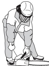
Grip the front handle with your left hand. Hold the chain saw on the ground by placing your right foot through the rear handle. Pull the starter handle with your right hand and pull out the starter cord slowly until you feel a resistance (as the starter pawls engage) then pull firmly and rapidly. **Never wrap the starter cord around your hand**
