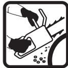
Never operate a chain saw holding it with one hand only. Please see page 30 in your "Chain saw operator's safety manual".
