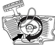
**CAUTION!** Check that the pulley can be turned at least a further 1/2 turn when the starter cord is pulled all the way out.
