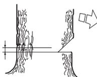
Use full throttle and bring the bar and chain slowly into the tree. Make sure the tree does not start to move in the opposite direction to your intended felling direction. Drive a wedge or breaking bar into the cut as soon as it is deep enough.
