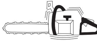
When you use a chain saw, vibration is generated by the uneven contact between the chain and the wood you are cutting.
