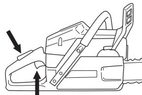
Push in the choke control as soon as the engine fire and make repeated starting attempts. Immediately press and release the throttle when the engine starts. That will disengage the throttle latch.
