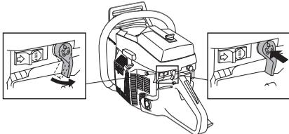
Note: It is not necessary to pump continuously. When the extra oil flow has been activated oil consumption increases by 40-80%, depending on the oil pump's basic setting.
