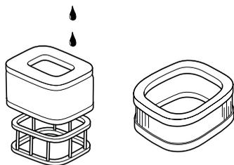
An air filter that has been in use for a long time cannot be cleaned completely. The filter must therefore be replaced with a new one at regular intervals. **A damaged air filter must always be replaced.**
