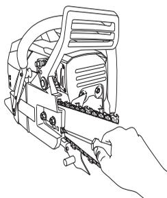
The chain is correctly tensioned when it does not sag from the underside of the bar, but can still be turned easily by hand. Hold up the bar tip and tighten the bar nuts with the combination spanner.
