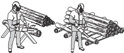
**The log is lying on the ground.** There is little risk of the chain jamming or the object splitting. However there is a risk that the chain will touch the ground when you finish the cut.
