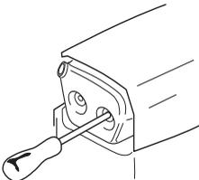
Some mufflers are equipped with a special spark arrestor screen. If your machine has this type of muffler, you
