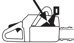
Move the front hand guard forwards and back to make sure it moves freely and that it is securely anchored to the clutch cover.
