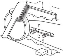
Regularly check that the brake band is at least 0.024 inch (0.6 mm) thick at its thinnest point.
