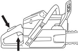
As the chain brake is still activated the engine must return to idling speed as soon as possible by disengaging the throttle latch in order to avoid unnecessary wear on the clutch assembly.
