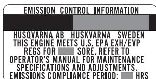
The Emissions Compliance Period referred to on the Emission Compliance label indicates the number of operating hours for which the engine has been shown to meet Federal emissions requirements.
