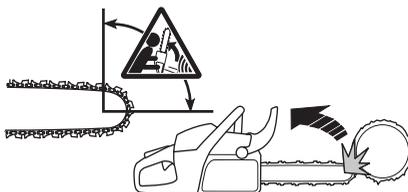
Cutting with the bottom edge of the bar, i.e. from the top of the object downwards, is known as cutting with a pulling chain. In this case the chain saw pulls itself towards the tree and the front edge of the chain saw body rests naturally on the trunk when cutting. Cutting with a pulling chain gives the operator better control
