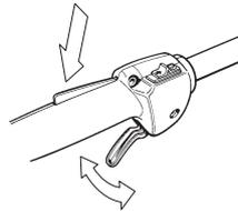
See instructions under the heading Start. Start the machine and apply full throttle. Release the throttle and check that the cutting attachment stops and remains at a standstill. If the cutting attachment rotates with the throttle in the idle position then the carburettor idle setting must be checked. See instructions under the heading Maintenance.
