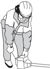
**CAUTION!** Do not put any part of your body in marked area. Contact can result in burns to the skin, or electrical shock if the spark plug cap has been damaged. Always
