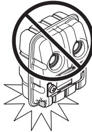
Regularly check that the muffler is securely attached to the machine.
