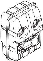
In countries that have a warm and dry climate there is a significant risk of fire. We therefore fit certain mufflers with a spark arrestor mesh. Check whether the muffler on your machine is fitted with this kind of mesh.
