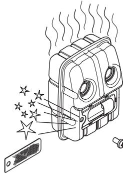
**CAUTION!** Never use a machine with a defective muffler.
