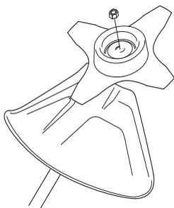
When fitting, tighten the nut in the opposite direction to the direction of rotation of the cutting attachment. To remove it, undo the nut in the same direction as the cutting attachment rotates. (CAUTION! The nut has a left-hand thread.)
