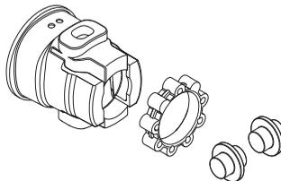
Regularly check the vibration damping units for cracks or deformation. Check that the vibration damping element is undamaged and securely attached.
