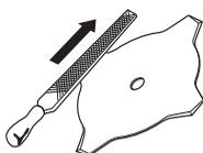
Check the cutting attachment for damage or cracks. A damaged cutting attachment should always be replaced.
