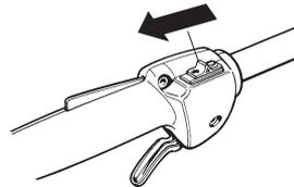
**Primer bulb:** Press the primer bulb repeatedly until fuel begins to fill the bulb. The bulb need not be completely filled.
