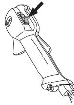
**Choke:** Set the choke control in the choke position.
