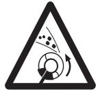
The operator of the machine must ensure, while working, that no persons or animals come closer than 15 metres.
