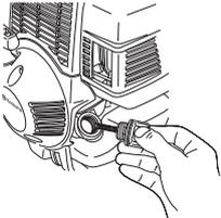
When the oil level is low, top up using engine oil to the edge of the oil refill hole.
