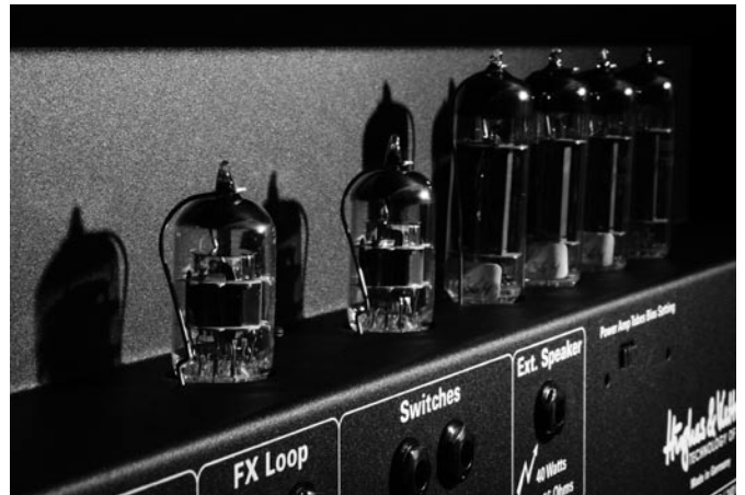
Illustration: QUAD EL 84, 2x 12AX7, 4x EL84
