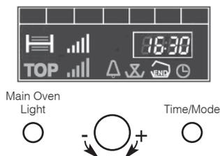
STEP 6. Press the Time/Mode button, until the 'end time' symbol is flashing. The display will show a default cooking end time (this will be the current time plus the cooking duration you set in STEP 5). The 'end time' symbol will flash.
