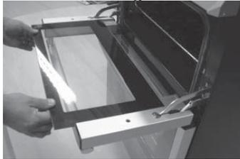
2. Carefully slide the inner glass towards you and withdraw it from its locating slots. Ensure that the door is not allowed to slam shut, due to the reduction in door weight. Clean the glass as described above.
