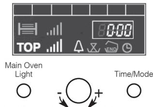
STEP 1. Press the Time/Mode button, until the 'bell' symbol is flashing.
