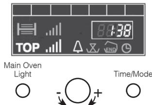
The minute minder can be cancelled at any time by following STEPS 1 and 2, setting the time period to zero using the +/- control knob. The display will revert back to the time of day.
