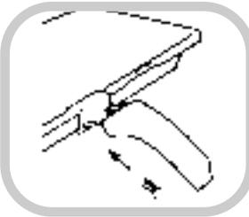
The grill pan handle is detachable from the pan, to facilitate cleaning and storage. The handle can be either detachable from or fixed to the pan. For a fixed handle remove the screw and washers from the grill pan bracket, tilt the handle over the recess adjacent to the bracket.
