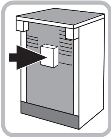
The control unit should be easily accessible in the event of an emergency, but must be within 2 metres of and not directly above an appliance.
