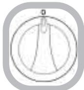
The controls set the hotplates at six pre-set power levels. Each control can be used to select one of six temperature settings from a minimum at position 1 to a maximum at position 6
