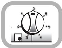
The controls set the hotplates at six pre-set power levels. Each control can be used to select one of six temperature settings from a minimum at position 1 to a maximum at position 6, the redspot hotplates heat up more rapidly to give faster boiling.
