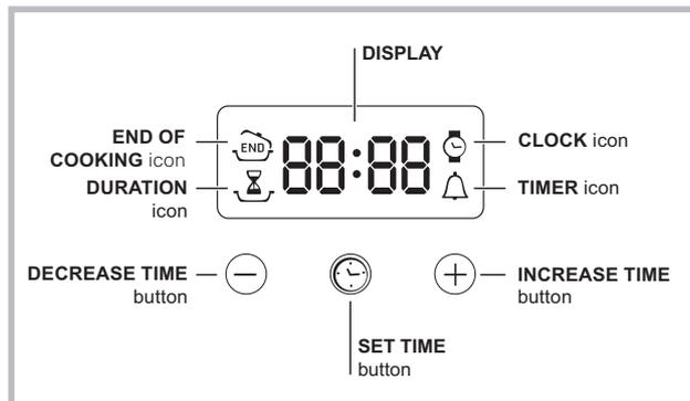
! The Top Oven and Main Oven can be controlled by the automatic timer. When the timer control has been set for one oven, it is possible to use the other oven only during the same automatic cooking programme.
