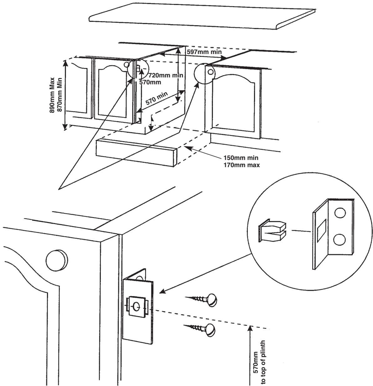
A minimum distance of 25mm should be maintained between the front face of the cabinet side and the front face of the plinth.
