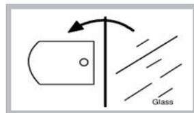
3. The inside of the outer door glass can now be cleaned while still fitted to the cooker.
