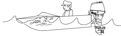
INCORRECT CAUSES BOAT TO “PLOW”
