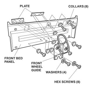
Reinstall the front bed panel and the upper tiedown hooks.
