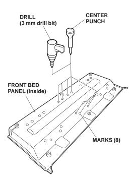
4. While wearing eye protection, enlarge the eight holes to 9 mm from the outer surface side of the front bed panel. Remove all burrs from the edges of the holes with a file.
