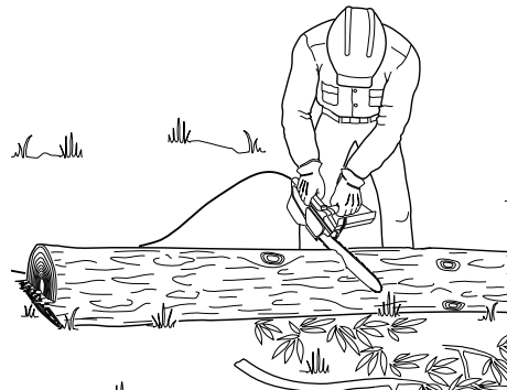
Figure 14 - Bucking Log With Entire Length On Ground
