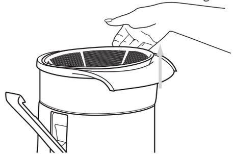
6. Lift the juice collector/bowl from the motor base – figure 12.
