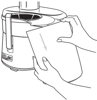
3. Place fingers under the bottom of the twin-locking handles and lift to release – figure 9.
