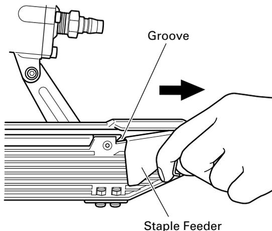
(2) Place the staple strip over the magazine. Make sure that the staple strip slides freely on the magazine.
