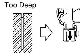
If the staple is driven in deeply, adjust the push lever piece to "down", and if it's driven in shallowly, adjust the push lever piece to "up".
