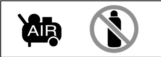
Never use oxygen, combustible gases or any other bottled gases as a power source for the Stapler.
