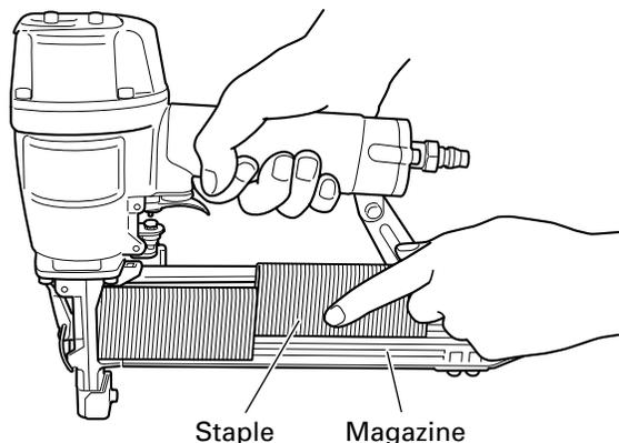
(3) Pull the staple feeder backward. Then, detach it from the groove of magazine and softly bring the staple back as if it were being gently pushed, avoiding any impact.
