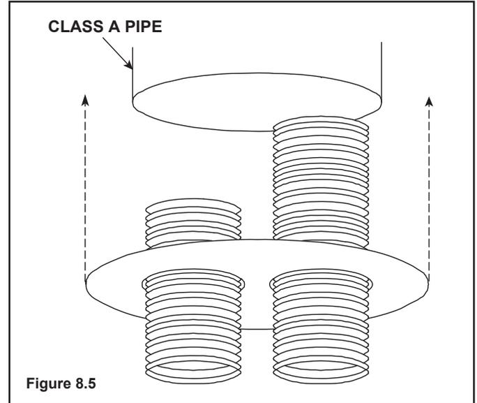
To prevent odors and cold drafts, the chimney must be sealed around the vent with non-combustible blanket insulation or field fabricated metal plates.
