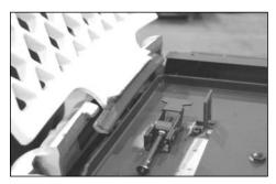
Figure 8.22 Gently lift cast top off of unit and set aside.
