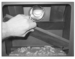
**Figure 8.4** Installation of the flue restrictor requires the removal of the baffle located inside the firebox. Remove the baffle by first removing the two screws holding the baffle in place (one on each side).
