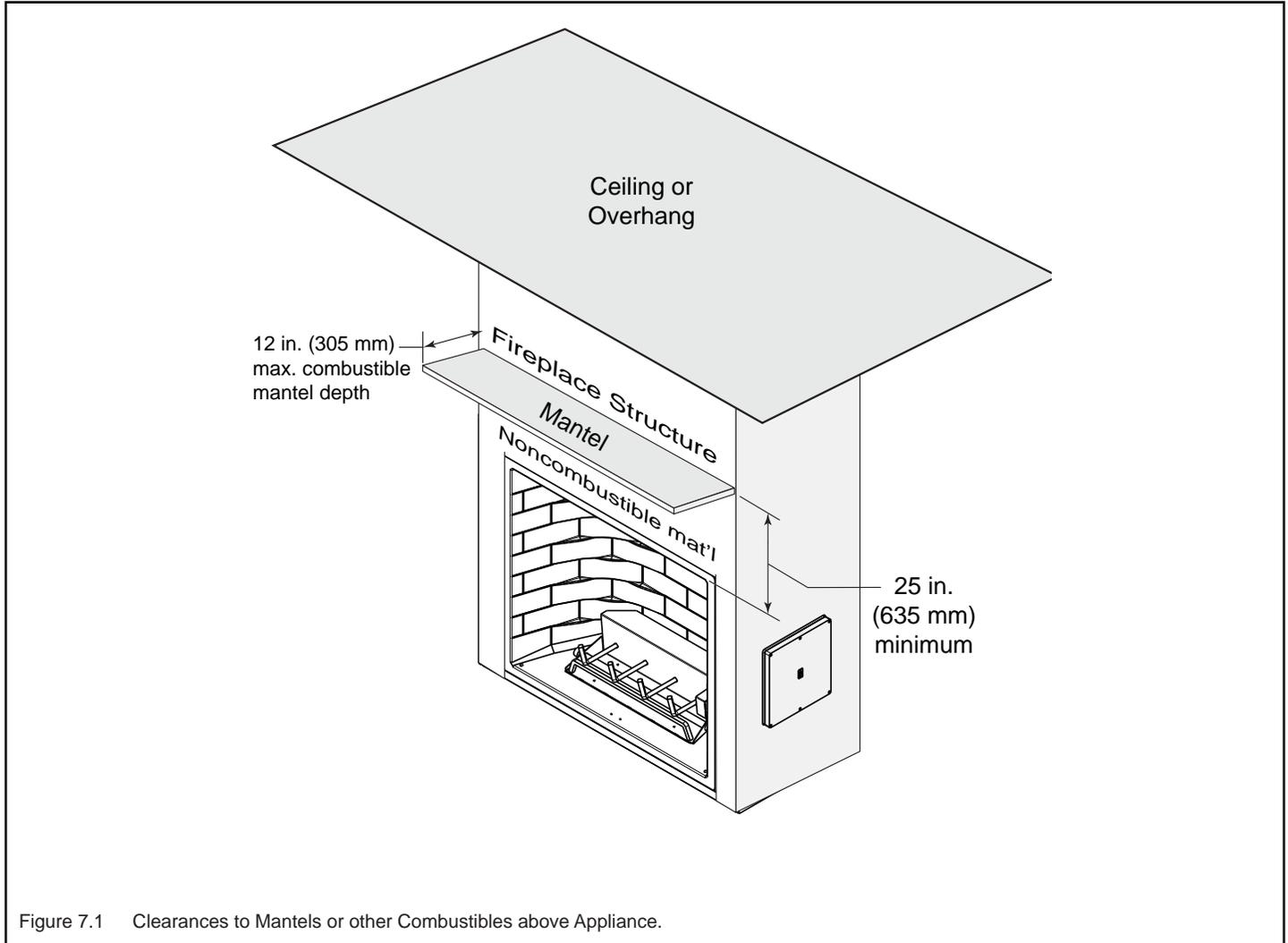
Figure 7.1 Clearances to Mantels or other Combustibles above Appliance.
