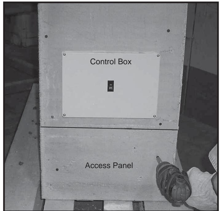
Figure 5.1 Control Box & Access Panel Locations
