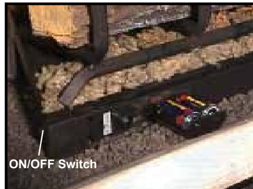
Figure 15 - Battery Replacement
