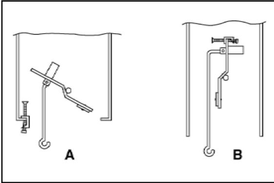
Figure 2 - Damper Operation
