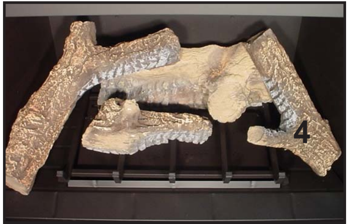
LOG #4 (SRV385-722): Place log #4 on 5th grate bar and rest its top into the groove on log #1.
