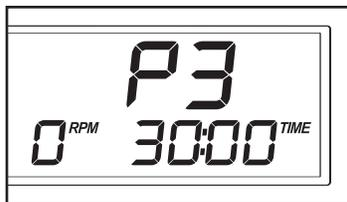
The diagrams numbered 1 through 4 on the right side of the console show how the resistance level will change during the resistance programs. For example, diagram number 3 shows that when program 3 is selected, the resistance will gradually increase throughout the program, and then decrease near the end.
