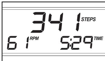
when you use the handgrip pulse sensor. The display will also show the resistance level for a few seconds each time the resistance setting changes. Note: When a resistance program is selected, the display will show the time remaining in the program instead of the elapsed time. To reset the display, press the On/Reset button.
