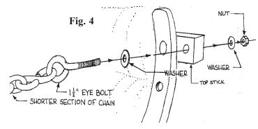
5. To attach the chain assemblies, work on one side at a time. On one of the chain-and-ring assemblies, find the shorter section of and-ring assemblies, find the shorter section of chain with an eye bolt. Place a washer on this eye bolt, and insert the eye bolt through the outside hole on one end of the top stick. Tighten using a washer, a nut, and a 9/16" wrench. (See Fig. 4)
