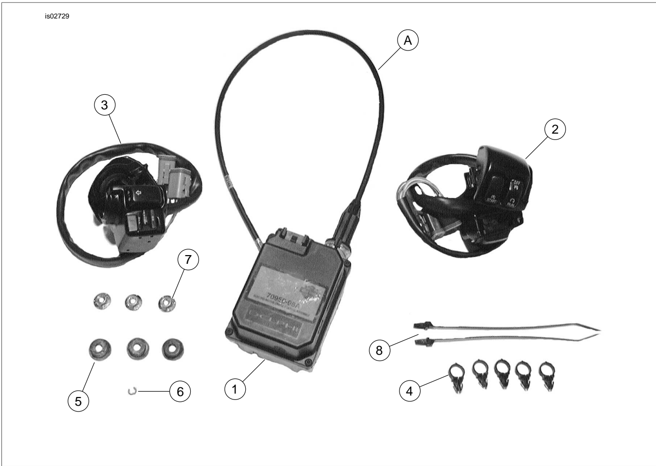
Figure 10. Service Parts: FLHR/I and FLHRS/I Cruise Control Kit
