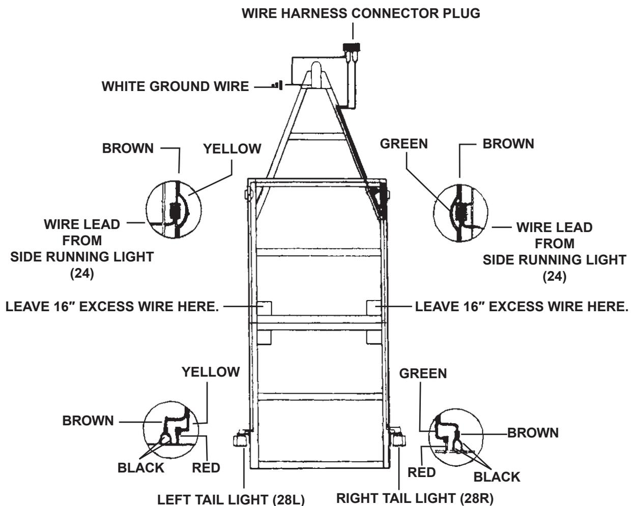
Figure J: Trailer Wiring
