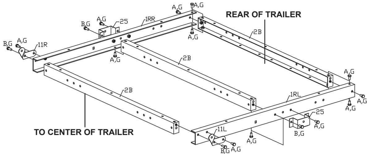
Figure C: Rear Bed Rail Assembly
