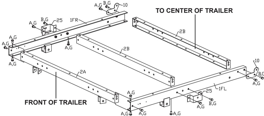
Figure A: Front Bed Rail Assembly
