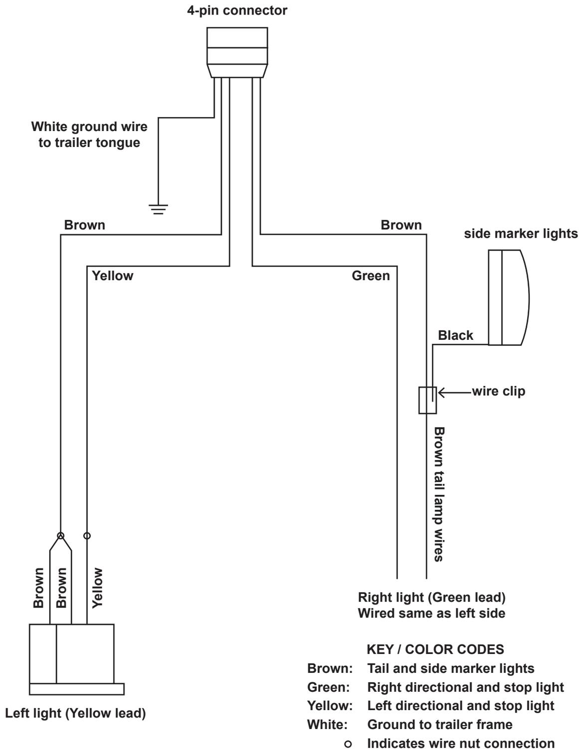
Figure K: Wiring Diagram
