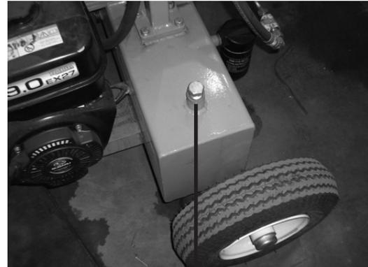
1. Remove the Hydraulic Oil Cap (20) and fill the tank with Hydraulic oil (not included) - See Figure F. Remove and retain the O-ring (21).
