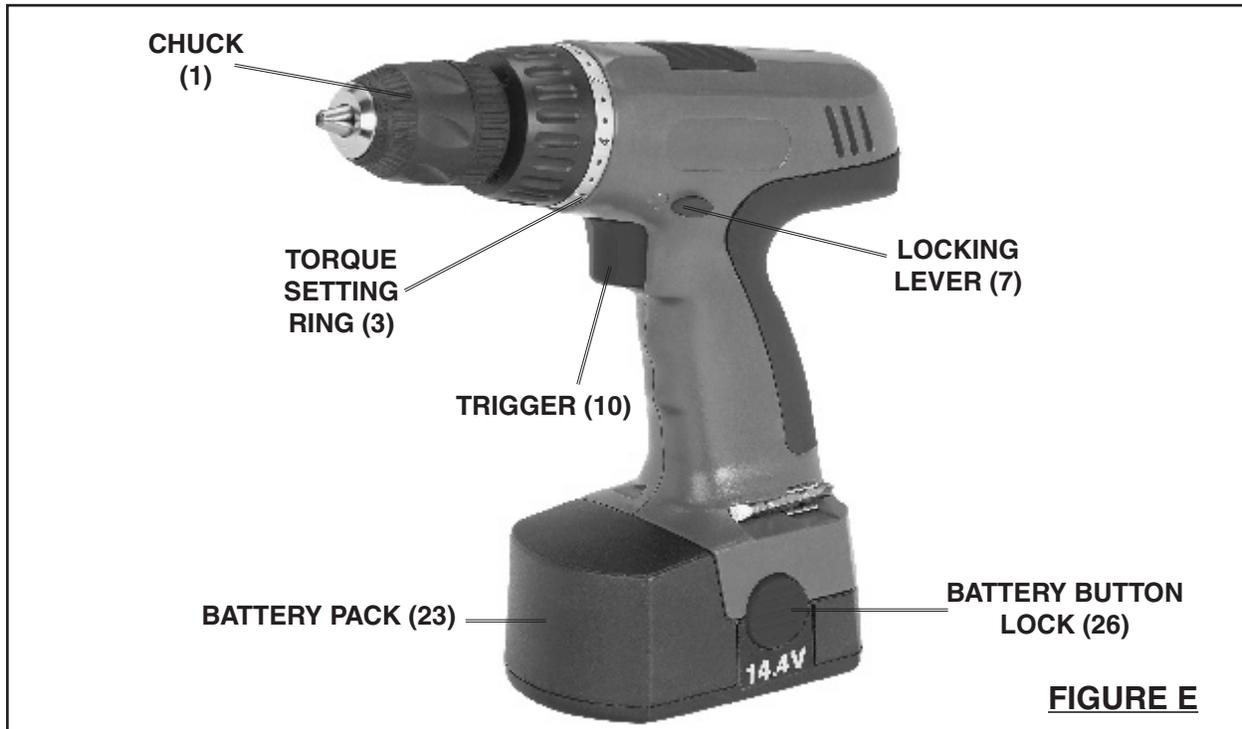
2. To install a drill/screwdriver bit, with the chuck pointing away from you, hold the Chuck Sleeve firmly in place and turn the Chuck (1) *counterclockwise*. Insert the shank of the bit all the way into the Chuck (1). While holding the Chuck Sleeve in place, turn the Chuck *clockwise* to lock the bit in place. The Chuck (1) accepts up to  $\frac{3}{8}$ " diameter bits. Insert the appropriate bit for your application and tighten the Chuck (1) firmly. **(See Figure E, above.)**
