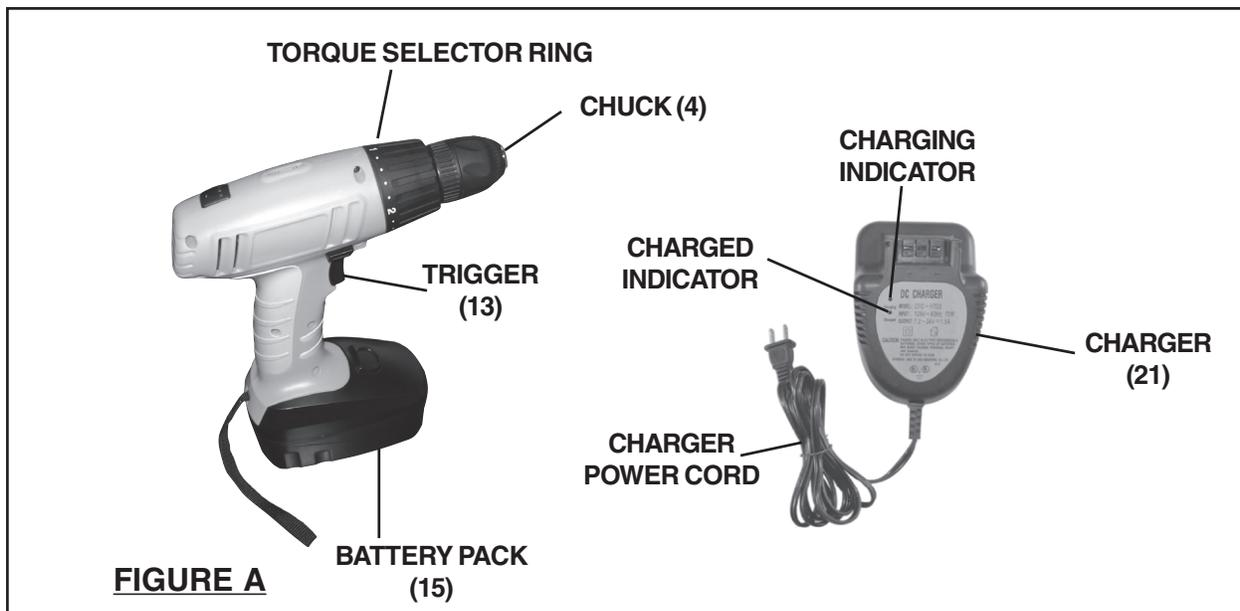
2. **Chuck (4):** Accepts up to 3/8" *shank* diameter Drill Bits (not included). To install a Drill Bit with the Cordless Drill pointed away from your body, hold the Chuck Sleeve firmly in place and turn the Chuck *clockwise*. Insert the shank of a Drill Bit all the way into the Chuck. While holding the Chuck Sleeve in place, turn the Chuck *counterclockwise* to lock the Drill Bit in place. **(See Figure A.)**
