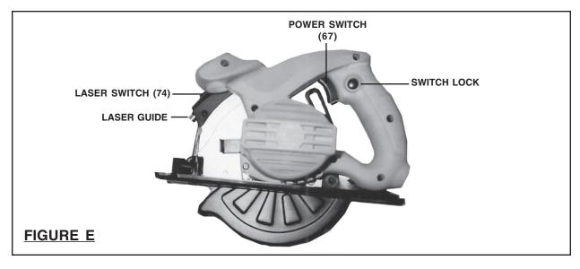
3. Laser Switch (74): The Circular Saw is equipped with a Laser Guide that is designed to aid alignment of the Saw Blade with the cutting line on the workpiece. To operate, push the Laser Switch to its "ON" or "OFF" positions. (See Figure E.)
