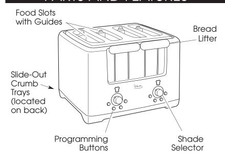
**Bread Lifter**—Push down the Bread Lifter to start the toaster. The Bread Lifter may be lifted up to stop toasting during a cycle.
