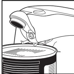
(Use the flip-up magnet to easily see can position.)
