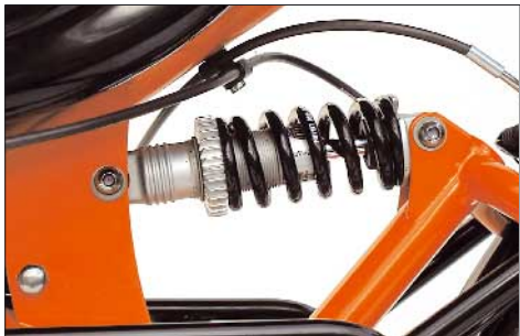
Suspension element DV-22 with fixed damping rate.
