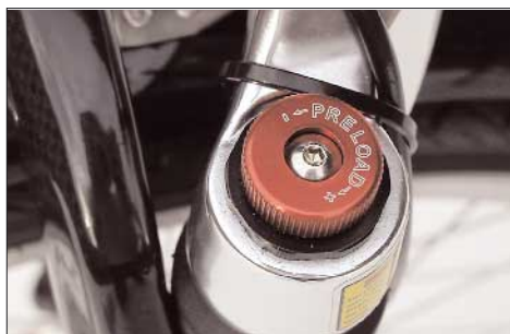
Turning knob for the pre-load of the suspension forks MEKS Carbon AC and MEKS Carbon All
