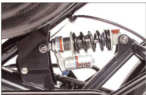
Suspension element ST8ARC with adjustable damping and piggy-back gas tank.
