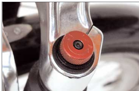
Turning knob for the pre-load of the suspension fork BALLISTIC XL-600All
