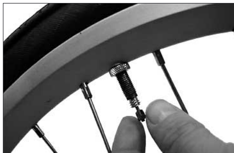
Before pumping up the tire, you have to undo the little knurled nut on the valve.
