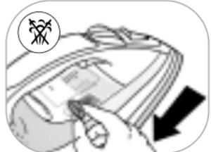
2. Open the cover of the water tank filler hole (C), place the iron on a table (not when iron is hot), as shown in the diagram, and then fill it.
