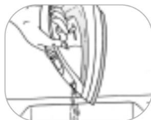
4. Wind the cord loosely around the heel and fix the clip (J) onto the cord.
