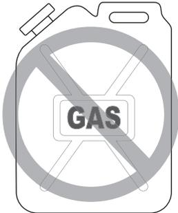
**Never clean this tool with gasoline or other flammable liquids. Vapors in the tool may ignite, causing the tool to explode. Ignoring this warning may lead to serious personal injury or even death!**
