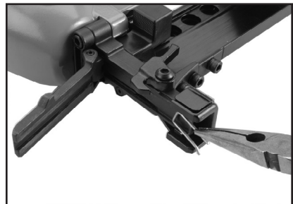
Figure 12. Removing a jammed staple.
