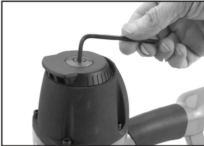
Figure 5. Loosening the exhaust cap screw.
