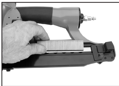
Figure 4. Loading a staple strip into the magazine.
