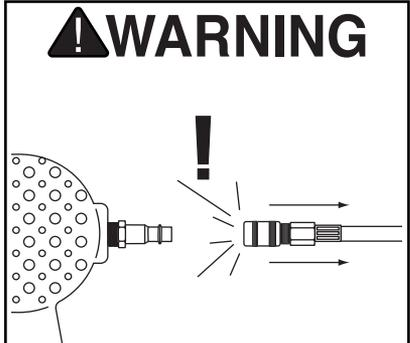
**Always disconnect air from stapler whenever servicing! During maintenance, a stapler connected to air may fire accidentally, causing serious personal injury!**
