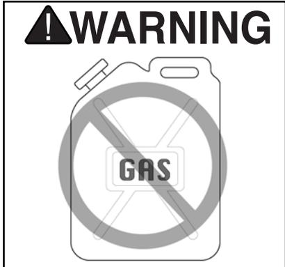
**Never use use gasoline or other flammable liquids to clean this tool. Vapors in the tool may ignite, causing the tool to explode. Ignoring this warning may lead to serious personal injury or even death!**
