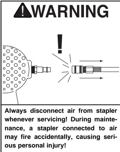
1. **Disconnect the stapler from the air supply!**
