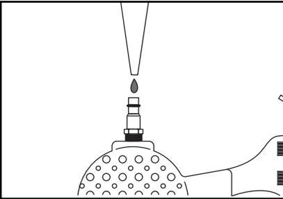
**Figure 5.** Lubricating stapler via air inlet.
