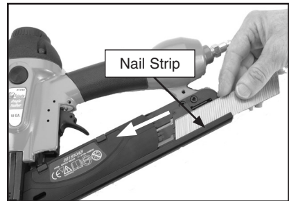
Figure 5. Loading a nail strip into the magazine.
