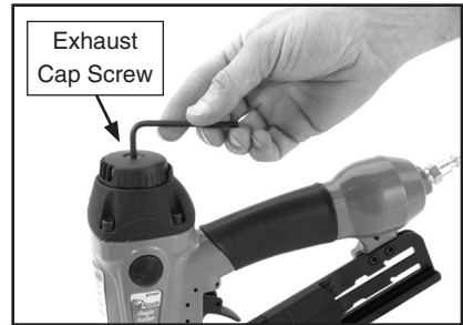
Figure 6. Loosening the exhaust cap screw.
