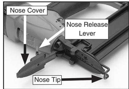
**Figure 7.** Nose opened to clear a jam.
