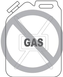
**Never use gasoline or other flammable liquids to clean this tool. Vapors in the tool may ignite, causing the tool to explode. Ignoring this warning may lead to serious personal injury or even death!**
