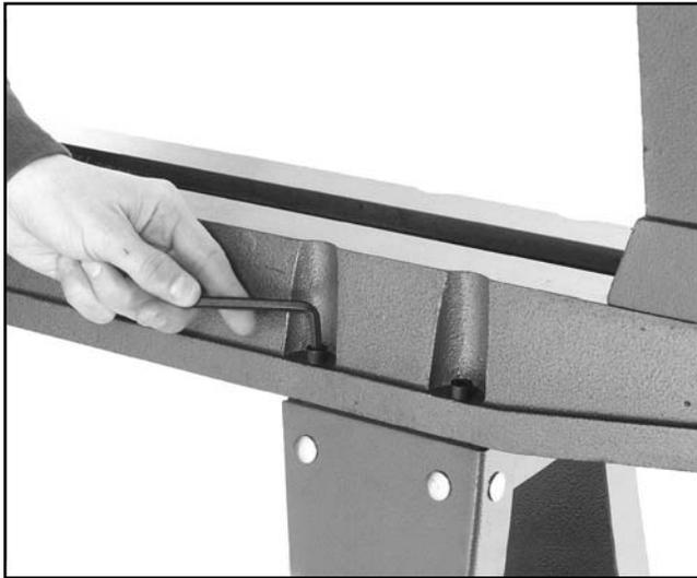
**Figure 5.** Attaching lathe unit to stand.
