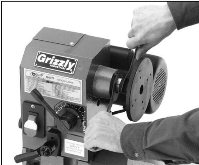
**Figure 10.** Attaching the faceplate.
