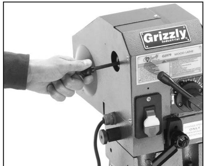
**Figure 9.** Removing the spur center.
