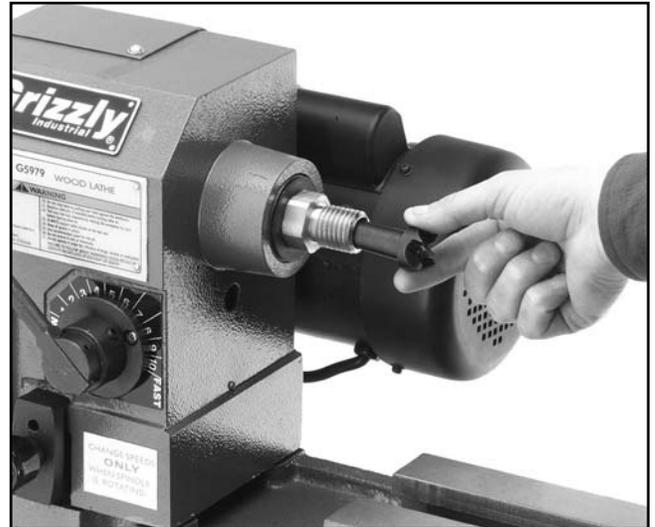
**Figure 8.** Installing the spur center.
