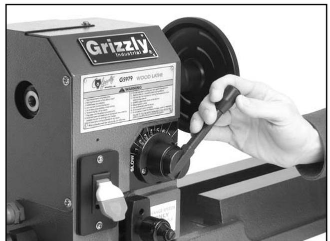
**Figure 16.** Adjusting spindle speed.
