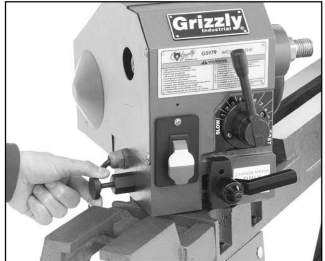
Figure 12. Adjusting headstock.
