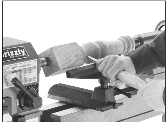
Figure 21. Proper hand positioning.
