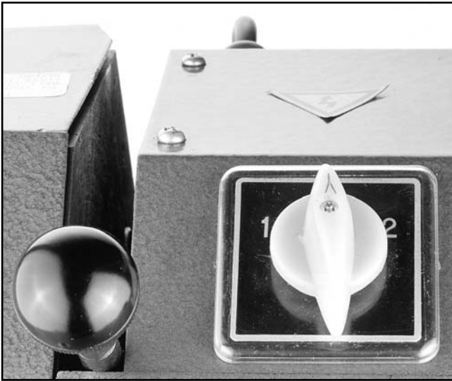
Figure 22. Power and directional switch.
