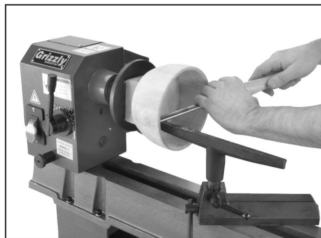
**Figure 38.** Typical faceplate turning operation.
