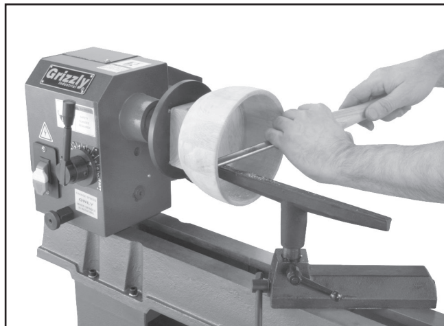
Figure 24. Typical faceplate turning operation.
