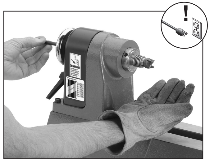
Figure 13. Removing spur center using the knock out bar.
