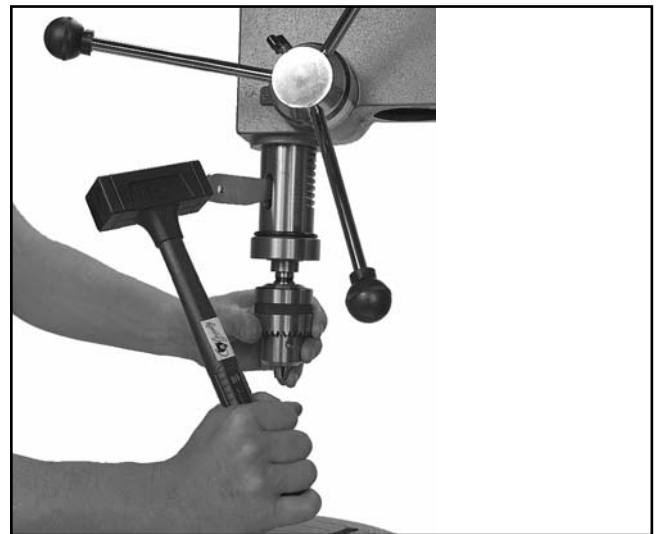
Figure 16. Removing the chuck.
