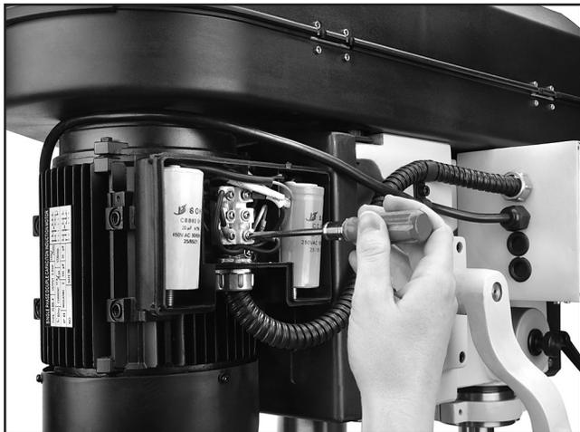
**Figure 9.** Changing motor jumper positions.
