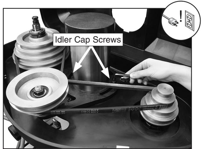
**Figure 31.** Pulley system.
