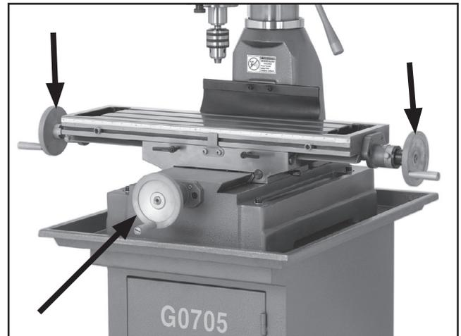
**Figure 20.** Table handwheel handles.
