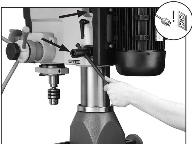
**Figure 40.** Headstock locking nuts.
